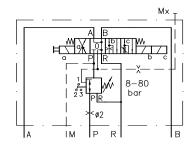
Switching position with fixed rapid traverse speed without pressure reduction and pressure monitoring.
