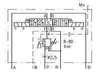
• Rapid traverse and creeping in one direction featuring also a limitation for rapid traverse (switching position a, c) rapid traverse in opposing direction (switching position b)
