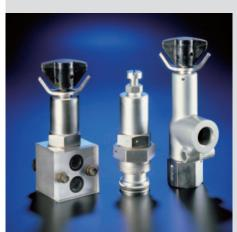
Directly controlled valves feature a dampening device to ensure quiet operation, but they are also available without it if necessary for an application. There is also a version of the pressure limiting valve (Type MV.X), conforming the Pressure Equipment Directive 97/23 EC, which features a type approval and a CE-stamping, usually necessary when used as safety valves for accumulators.
